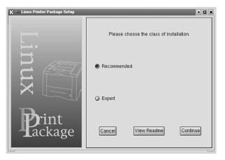
**Recommended** is fully automated and is not required any interaction. **Expert** installation allows you to select the install path or printing system.
